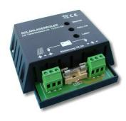
As a result of a late development, the PSX solar chargers appeared among our existing solar charge controllers with high expectations. The range currently consists of two models, the PSX182 (6A) and the PSX199 (8A), both regulators are made using highly reliable SMD components.
